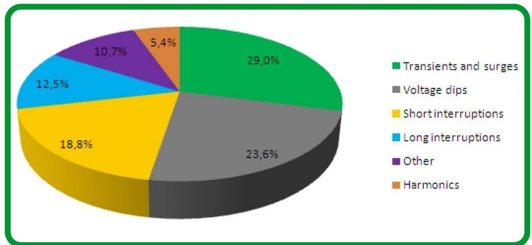
Each facility has its own specific power quality issues, depending on the installed loads, equipment, and the quality of supplied energy. However, based on the above international survey results and the rich group experience of hundreds of power quality audits and analyses realized every year around the globe, we recommend the systematic monitoring of the following power quality problems:
