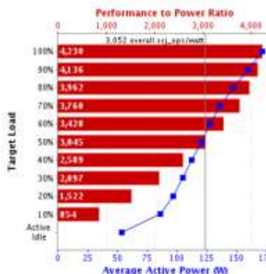
Servers consume a significant amount of power when they are idle, often more than 50% of peak power. As shown above, moving from 10% load to 50% load delivers 5x the performance for 40% more power.
