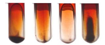
These test tubes contain untreated four months old fuel that was "aged" by a heating process. These samples from around the county, show variation in fuel stability.
