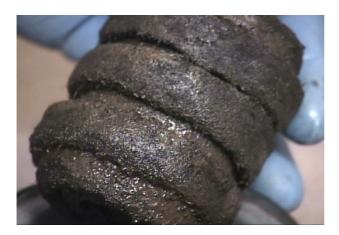
Increasing incidences of sludge in today's heating systems is a direct result of changes in the refining process.
