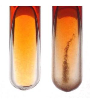
Although re-polymerization begins at a sub-microscopic level, as long-chain hydrocarbons begin to re-form they agglomerate and form visible sediment. The sample on the right shows the result of this process. The sample on the left was treated with a stabilizer and dispersant to inhibit re-polymerization.
