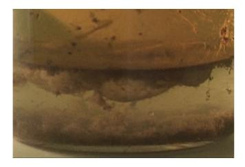
Bacterial, fungal or algae growth may occur. Even though performance problems due to microbial activity are less common than those resulting from re-polymerized fuels.
