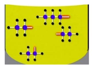
Active ends (shown in red) of artificially cracked hydrocarbon chains are the source of instability in today's fuels. Over time, these ends recombine, forming agglomerations of long chain molecules in stored fuel.
