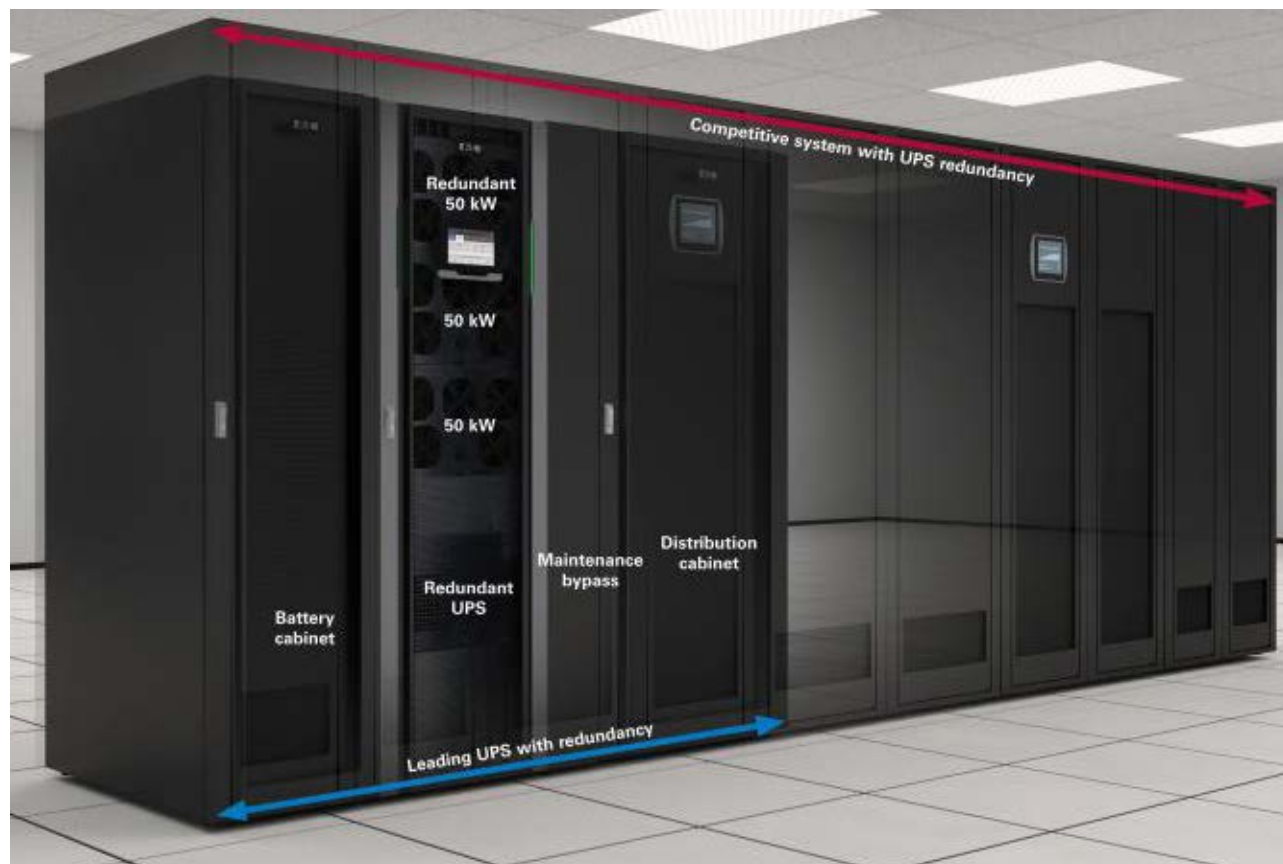
Figure 1. Modular UPSs save money and floor space by enabling data centers to “grow vertically” (reducing horizontal sprawl as shown above) and leverage internal redundancy, rather than install backup units.
