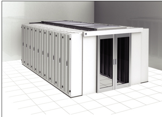
Figure 5: Standard Cold Aisle Containment Solution from CPI. In the example above, CPI Aisle Containment Doors are combined with an overhead ceiling and the F-Series TeraFrame® Cabinet System to enclose the cold aisle between adjacent cabinet rows. The overhead ceiling traps cold air in the aisle so that it will be used to cool equipment, instead of the entire room.
