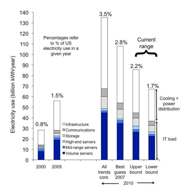
Figure 2: US electricity use for data centers (2000, 2005, and 2010)
